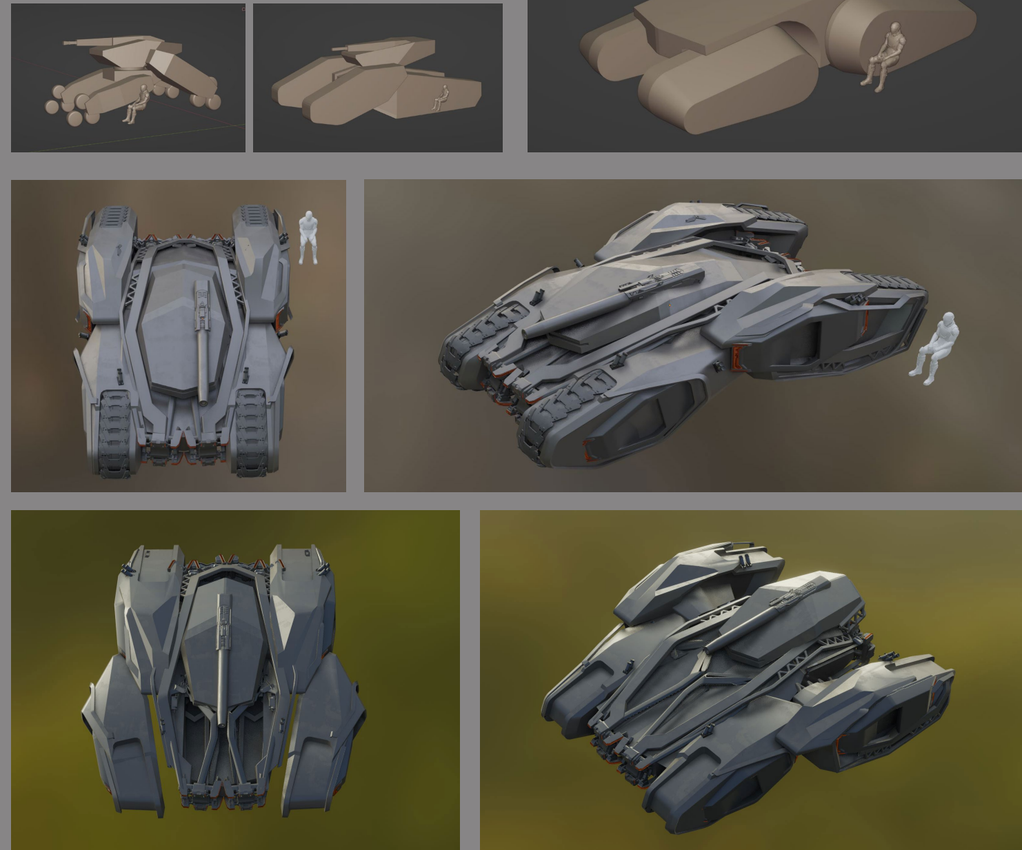
'Concept A' focused on a centrally mounted cannon with four separate tracks at each corner. Various track positions were considered, though the flat and wide shape was a constant.
